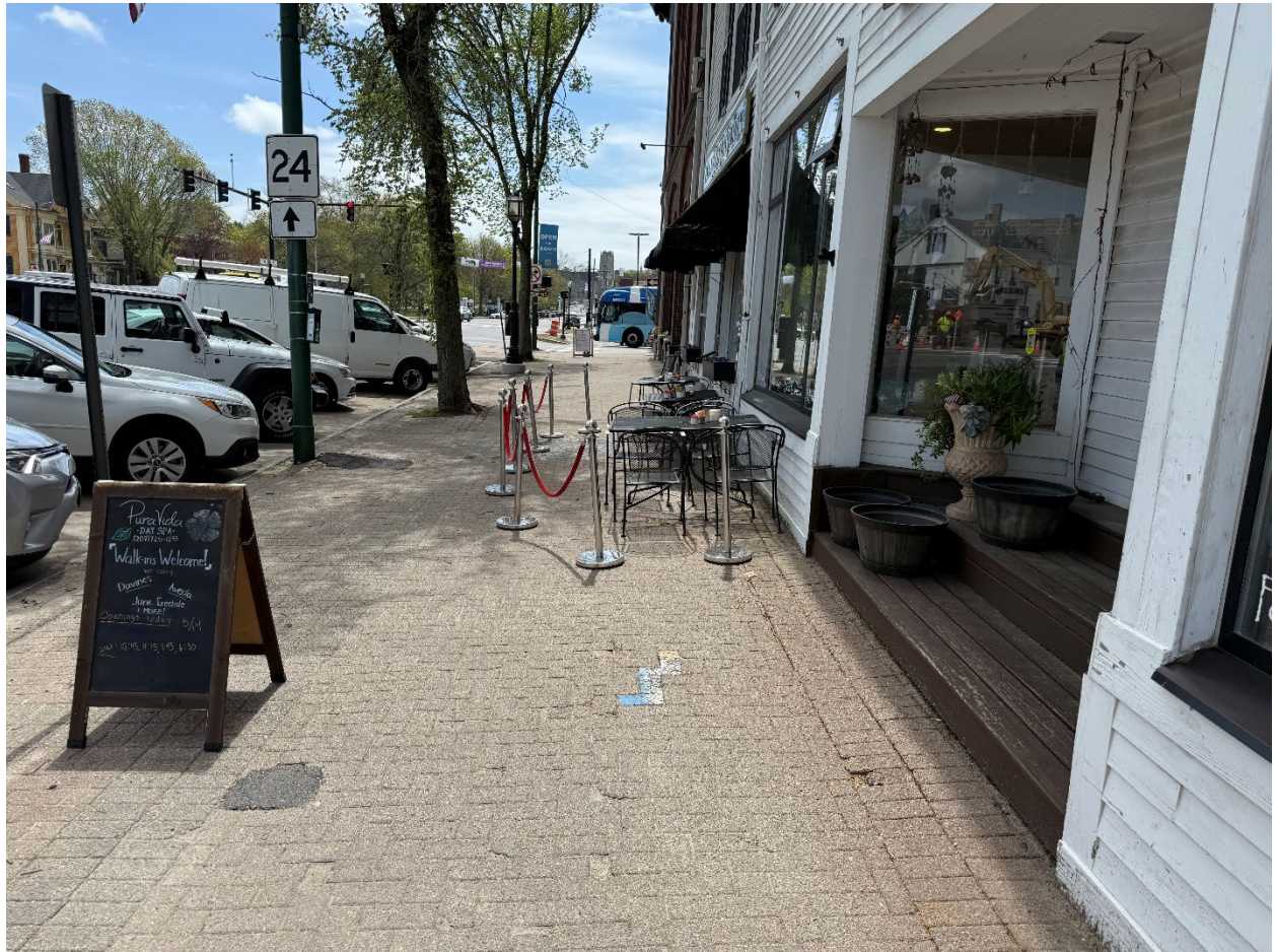
Note limited width of sidewalk to accommodate an ADA compliant path, outdoor dining area, and outdoor signage.
