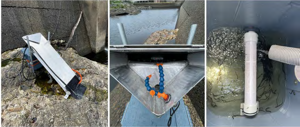
Figure 4-1: Images of the Temporary Eel Ramps Manufactured by Lakeside Engineering and Installed Downstream of the Project During the Visual Surveys of Upstream American Eel Movements Study Showing Installed Set-up (left image), Refresh and Conveyance Flow Nozzles (center image) and Holding Tank (right image).
