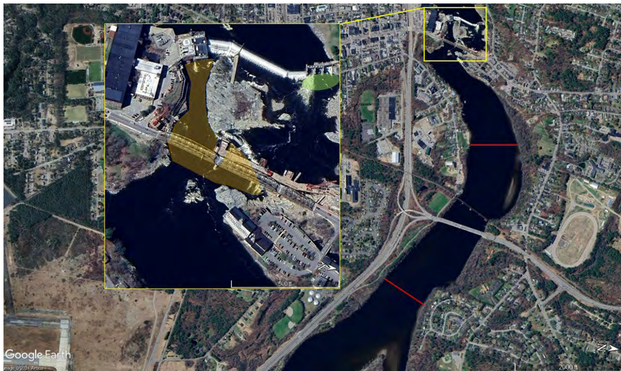
Figure 6–1: Relative Locations of Sampling Regions Identified in the RSP for Assessment During Phase I: Primary Detection Zone (Orange Shading; 2D Data Acquisition), 1D Spillway Region (Green Shading), and Gate Receivers (Red Line)
