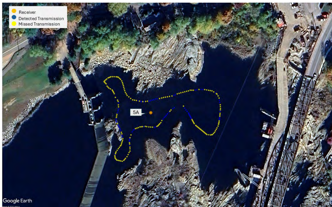
Figure 5–10: Receiver Placement and Locations of Recorded (Blue) and Missed (Yellow) Test Tag Transmissions During the Boat-Based Field Evaluation at Pilot Deployment Location 5 During Phase I of the Project Interaction Study at Brunswick
